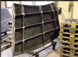
Red Bull Arch | Production 84 cast aluminium parts ca. 2x2m
