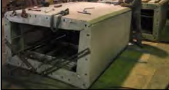
Red Bull Arch | Production 84 cast aluminium parts ca. 2x2m
